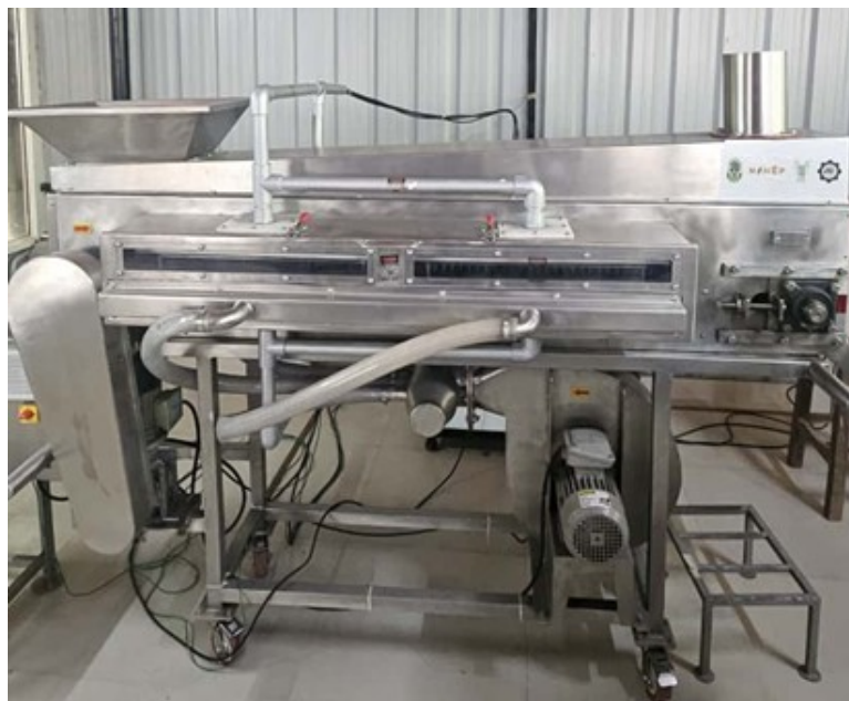
Figure 1: Dielectric barrier discharge (DBD) type Cold plasma apparatus
